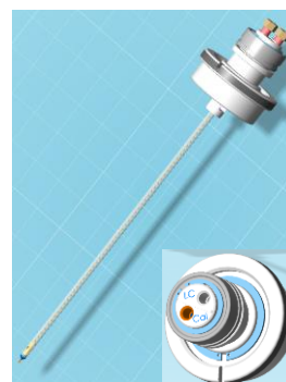
Figure 3. TwinSprayer ESI Probe. The unique design provides an independent flow path for calibration solutions, for easy maintenance of mass accuracy during LC-MS runs.
