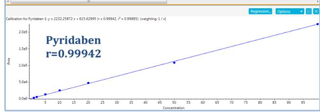
Figure 6 Quantitative linearity using pyridaben as an example
