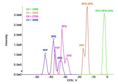
**Figure 2. Differential Mobility Spectrometry Resolves Isobaric Overlap.** The separation of 3-phosphoglycerate (3PG), 2phosphoglycerate (2PG) and phosphoenolpyruvate using SelexION technology was tested using four different separation voltages (SV). Using isopropanol as a modifier reagent, high SV voltages were effective in resolving all metabolites.
