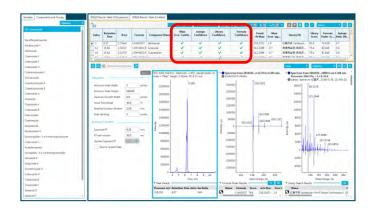
SCIEX OS software lets users filter results and display only those compounds meeting acceptance criteria and falling within confidence intervals defined by the user. It can quickly find targeted results in large databases.
