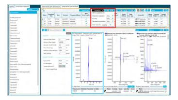
The TCM database of MS/MS spectra allows for secondary matching and yields more reliable results (grey color in the database indicates MS/MS data).
