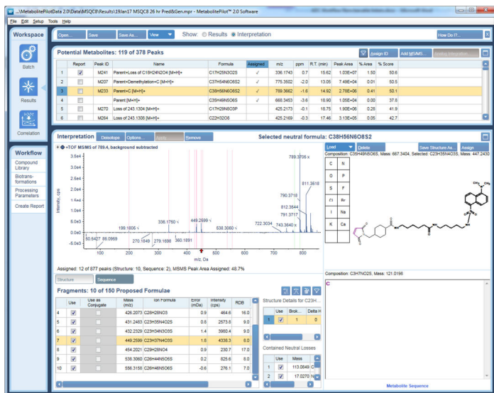
Figure 5. The interpretation results workspace of MetabolitePilot™ 2.0 software displaying results of the released payload species (payload+linker+cysteine) from the incubation of MSQC8 with human liver lysosomes. There are 3 product ions with proposed structures assigned to the payload species that include the dansyl fluorophore: 449.2599, 432.2329 and 336.1750.
