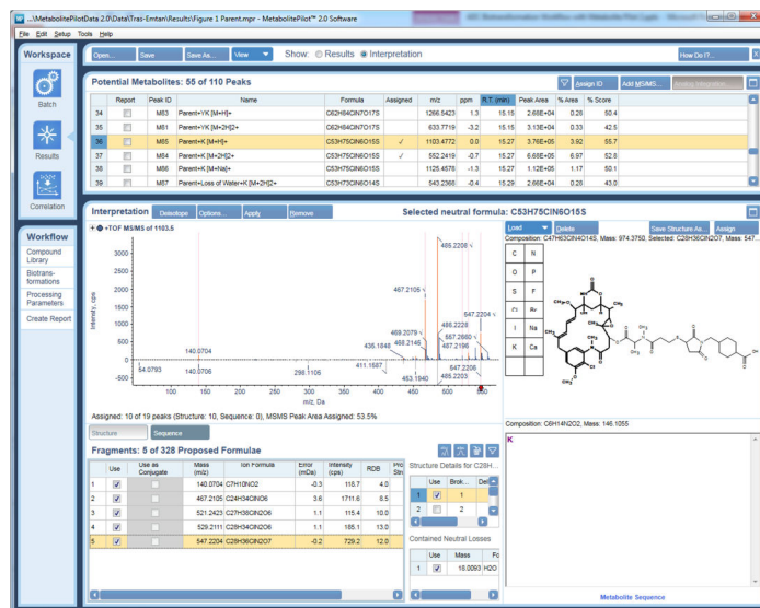
Figure 4. The interpretation results workspace of MetabolitePilot 2.0 software displaying results of the released payload species (payload+linker+lysine) from the incubation of T-E with human liver lysosomes. In this workspace product ions in the MS/MS spectra are assigned to the identified metabolite. There are separate assignments for both the small molecule payload and sequences of the mAb.
