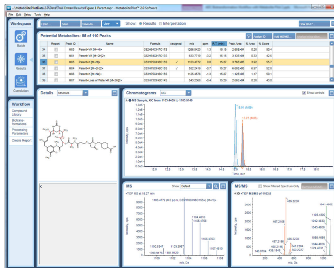
Figure 3. The results workspace of MetabolitePilot 2.0 software displaying results from the incubation of T-E with human liver lysosomes. The released payload species (payload+linker+lysine) was found at retention times 15.01 and 15.27 minutes as a pair of diastereomer peaks. The structure of the payload and linker species is displayed on the left with the amino acid of conjugation below. Also displayed is the MS and MS/MS spectra of the released payload species.
