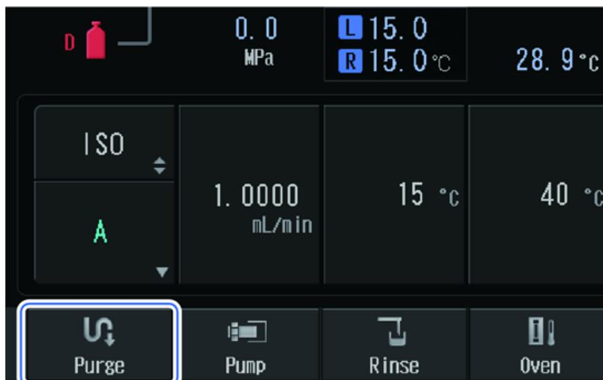
3. Turn ON **1st** to **4th** and **Rinse**. Keep the default purge time. Replace the entire flow line with mobile phase before setting the column.
