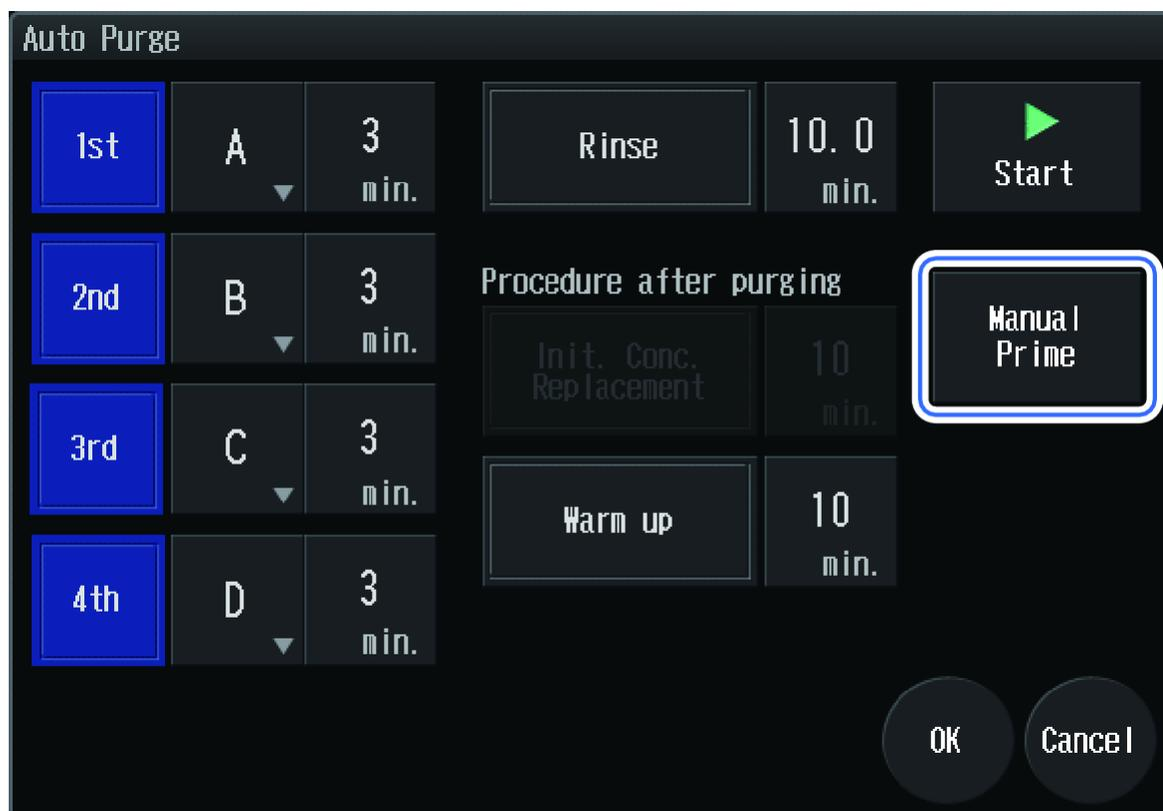
The flow line switches for manual priming.
