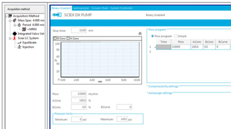
2. Edit the LC pump method as required for the experiments.
