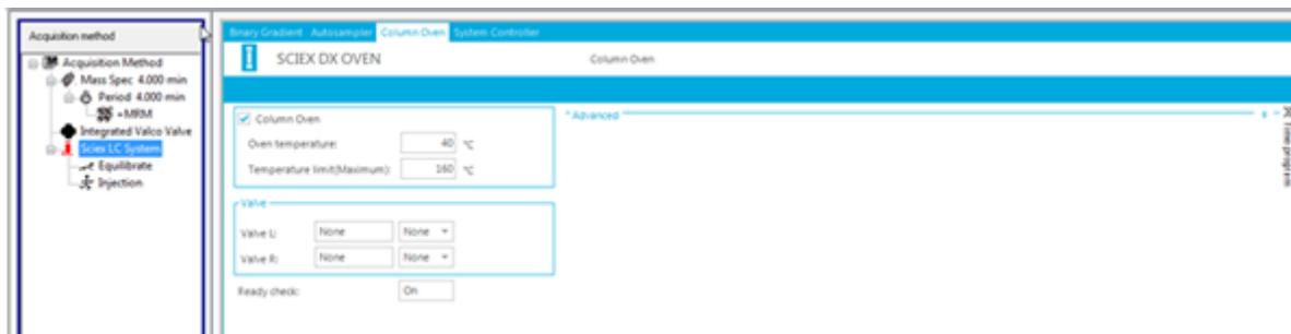
2. Type the temperature of the column oven or column oven compartments in degrees Celsius.
