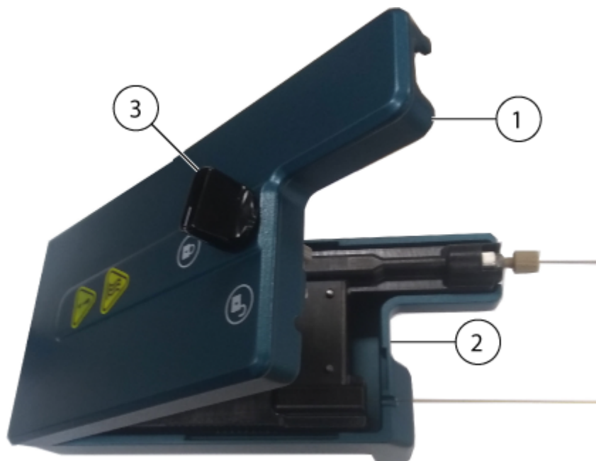
Figure 3-18 Front and Back Parts of the Nano Column Heater
