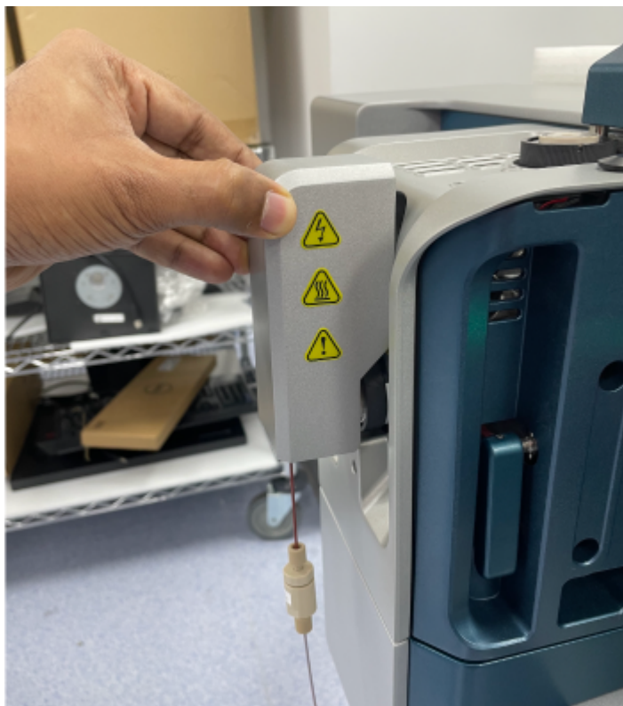
Figure 3-29 Protective Cap On the T-Fitting
